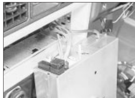
25.2b Removing the radio from its aperture
