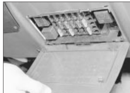
3.1 Removing the cover from the fuse/relay box
