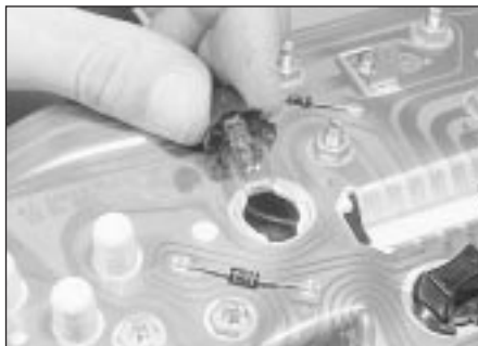
11.27 Removing an instrument panel bulb
