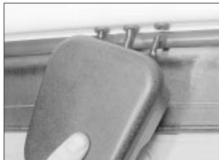
21.9 Removing the window-mounted motor
